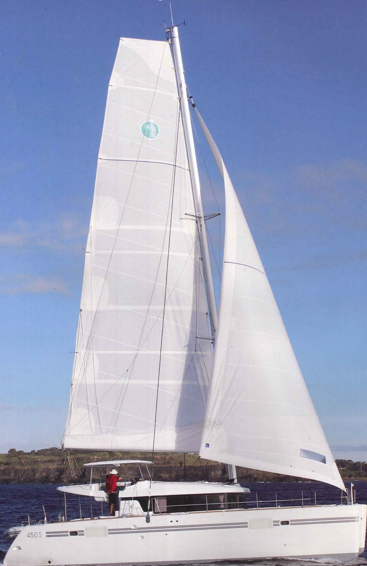
The Lagoon 450 S uses the same 45-foot hull as the original model but has an elevated helm, rather than a flybridge.
